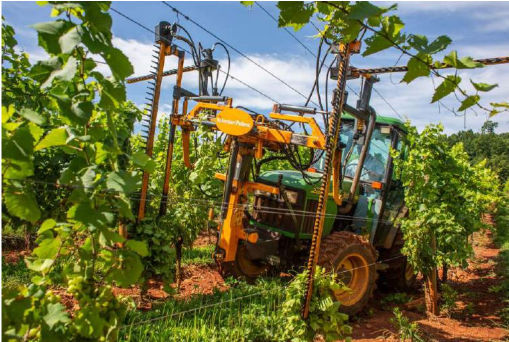
Francisco Ruiz drives a hedger, a machine that cuts leaves off the vine to clear the canopy for grapes, through the vineyard at Barboursville on Friday, July 21, 2023.
