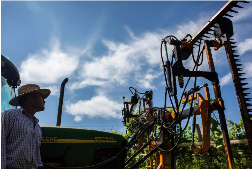
Francisco Ruiz looks at a hedger, a machine that cuts leaves off the vine to clear the canopy for grapes, at Barboursville Vineyards on Friday, July 21. CAL CARY photos, THE DAILY PROGRESS
