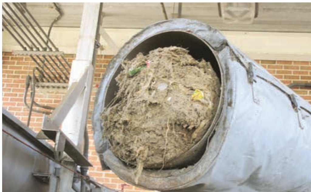
The compacted "leftovers," solid materials removed from wastewater, like plastics, fabrics and fast food wrappers.
