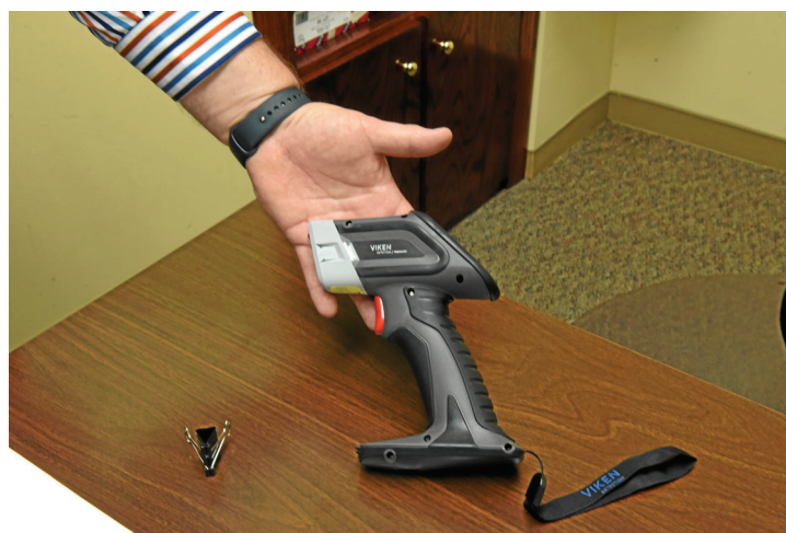
Danville Lead Safe Program Manager Michael Beckner shows the X-ray fluorescence lead-testing gun at his office Thursday morning.
