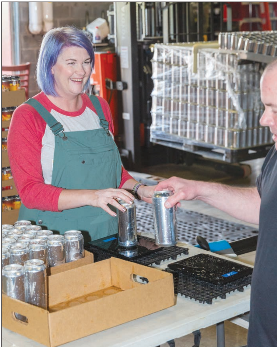
Holly Redding, owner and founder, Winchester Brew Works, weighs cans of lager to ensure the proper amount is in each can. PAUL LARA | INSIDENOVA
