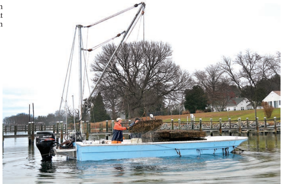
This 31-foot garvey was built to work in the oyster cage aquaculture business by Myles and Andy Cockrell. Photo by Larry Chowning
