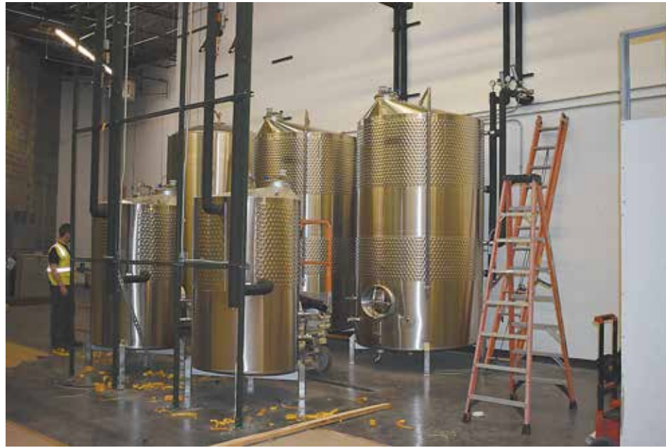
Left: Four of the tanks in the cidery's "tank farm" are fermenters for the ciders, while one of them force carbonates them. Right: Wright's mother, a master gardener, helped him plant eight apple trees in front of the cidery. Having the "orchard" out front allows Wright to operate the space as a farm winery with a tasting room.
