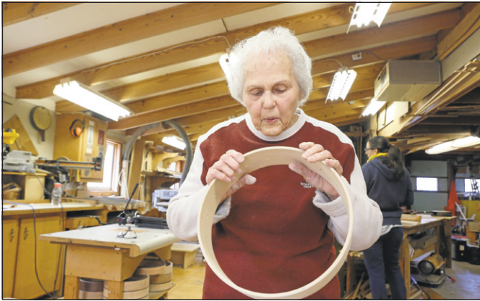
Kemp blows off sawdust after drilling pin holes in the rim.
