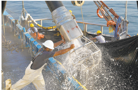
Engineer Julio Silva moves a giant vacuum hose used to gather menhaden from a seine net.
